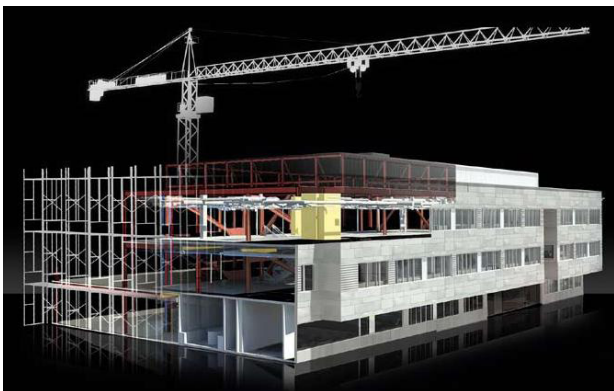
Figure 5. Building of the 4D model of the interactive Method of Statement for the modular building erection works as the basis for the creation of the 5D model based on BIM technologies
