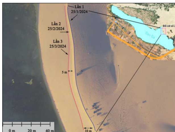
Fig. 3. Movement of the sand dunes during three surveys of the Trinh Nu hill
