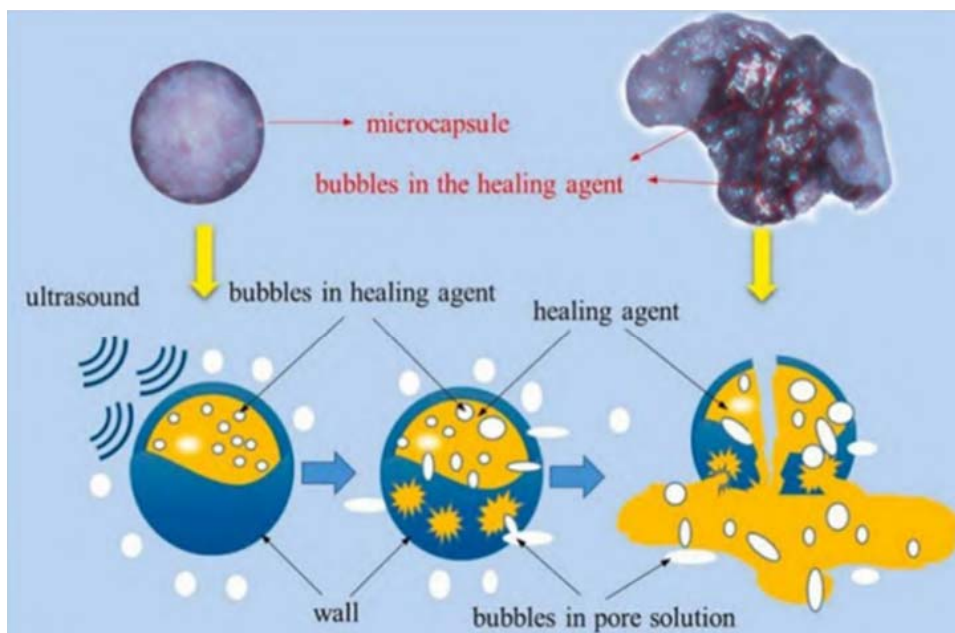
Fig. 5. Mechanism of ultrasound-induced rupture of microcapsules (Xu et al., 2018)
