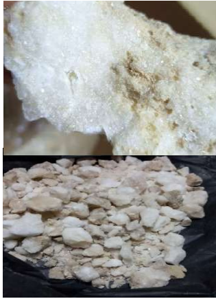
Fig. 2. Broken karshif stone (researchers' work)
