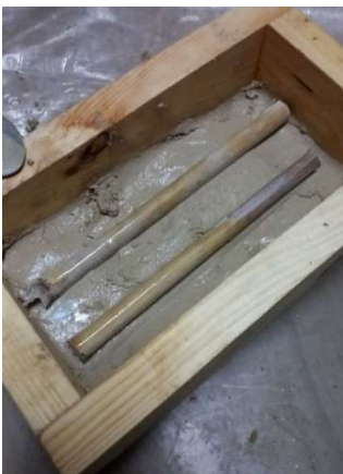
Fig. 3. Bamboo reinforcement visible within the brick sample (researchers' work)
