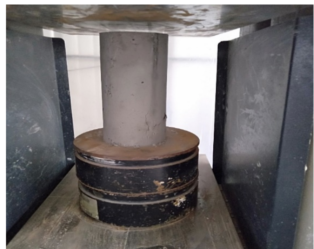
Fig. 5. Cylindrical specimens (100 × 200 mm) for compressive strength testing
