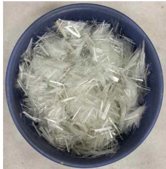
Fig. 4. Glass fiber reinforcement
