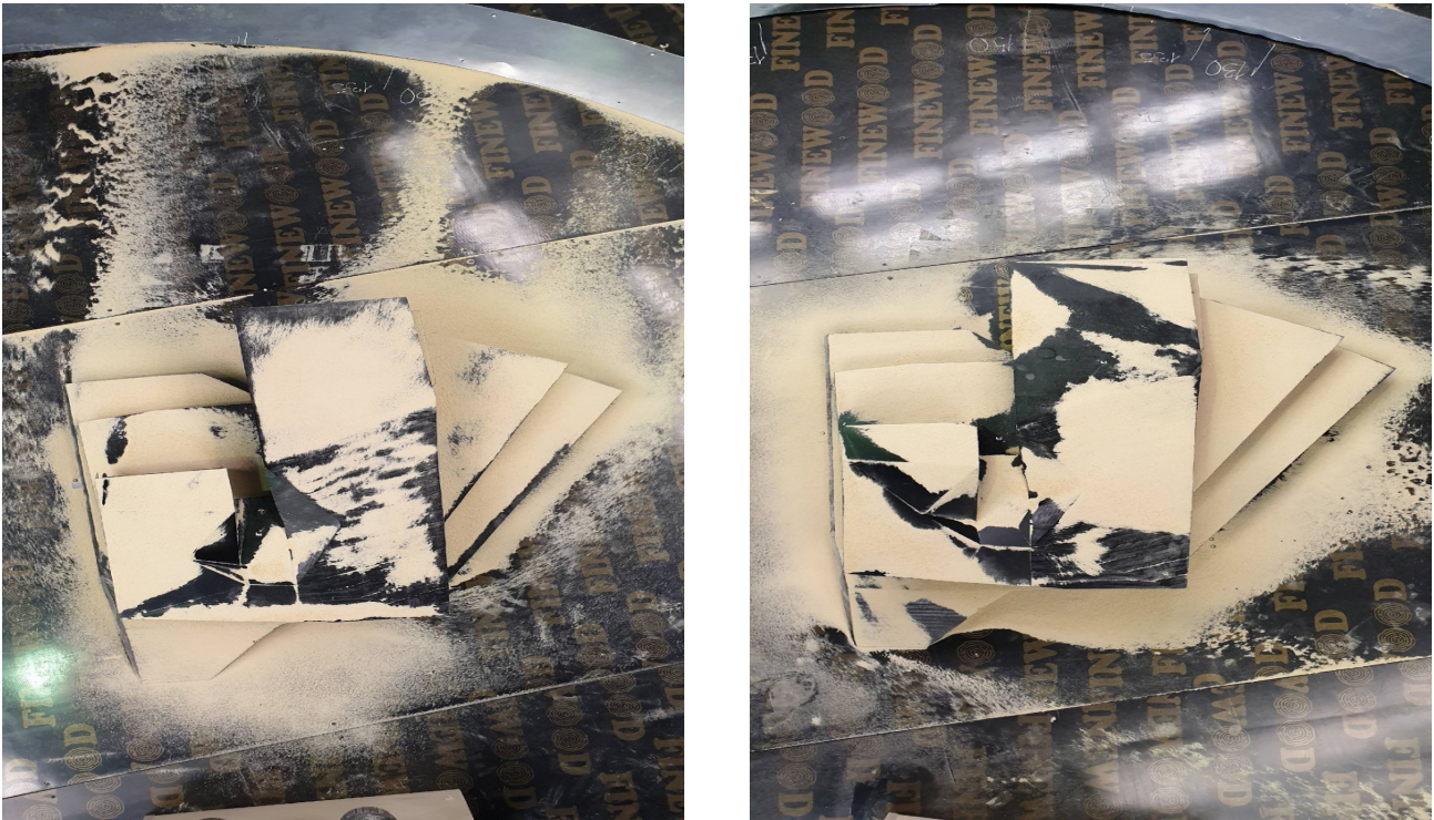
Fig. 5. Characteristic areas of snow deposits, wind angles 315° (NE) and 225° (SE)
