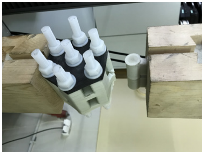
Fig. 12. Node after the tensile test
