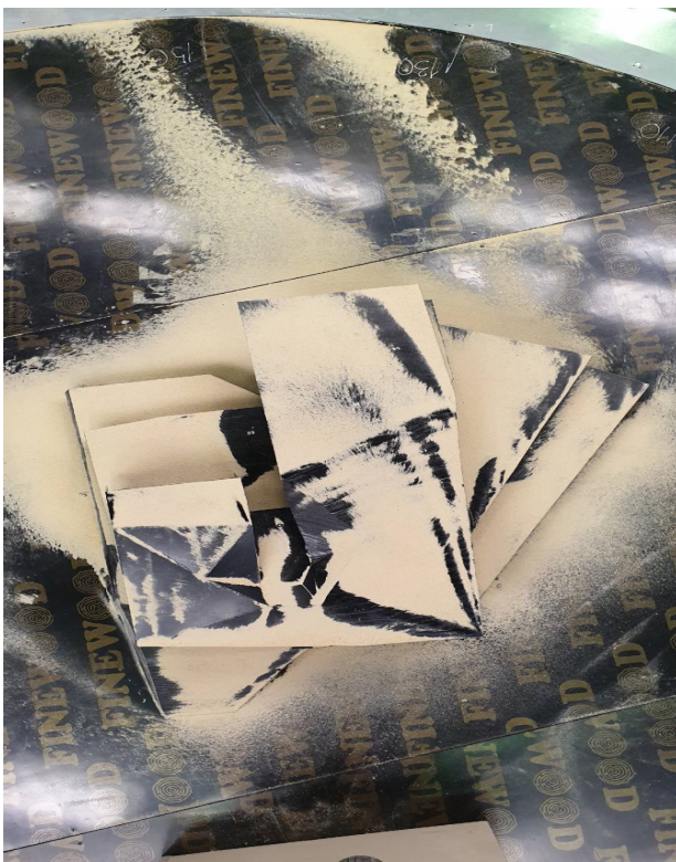
Fig. 4. Characteristic areas of snow deposits, wind angles: 0° (N) and 270° (E)
