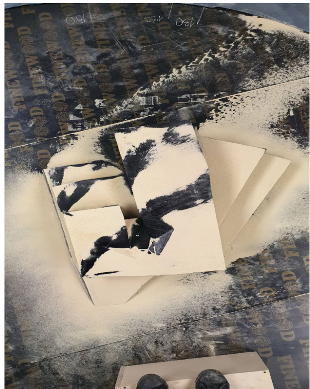
Fig. 4. Characteristic areas of snow deposits, wind angles: 0° (N) and 270° (E)
