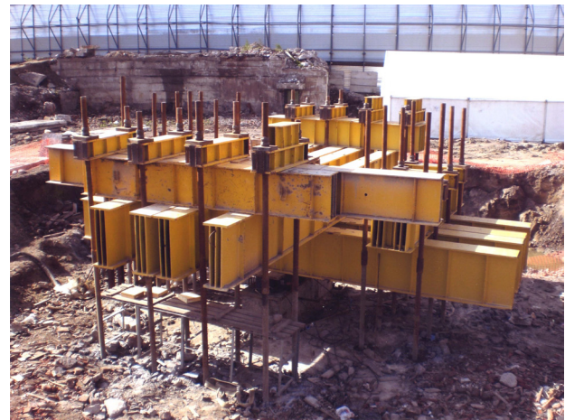
Fig. 1. General view of the loading platform for testing the piles with vertical static loading
