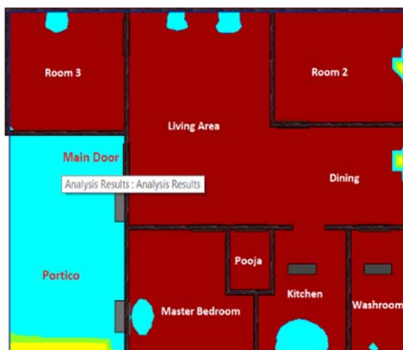
Fig. 5. Existing building illuminance
