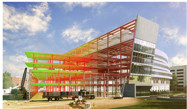
Figure 6. BIM data imported into GIS combined in the common 5D model (coordinates, time, movement) of construction and erection works execution with the possibility of movement across a facility and imbedded into «visual environment»
