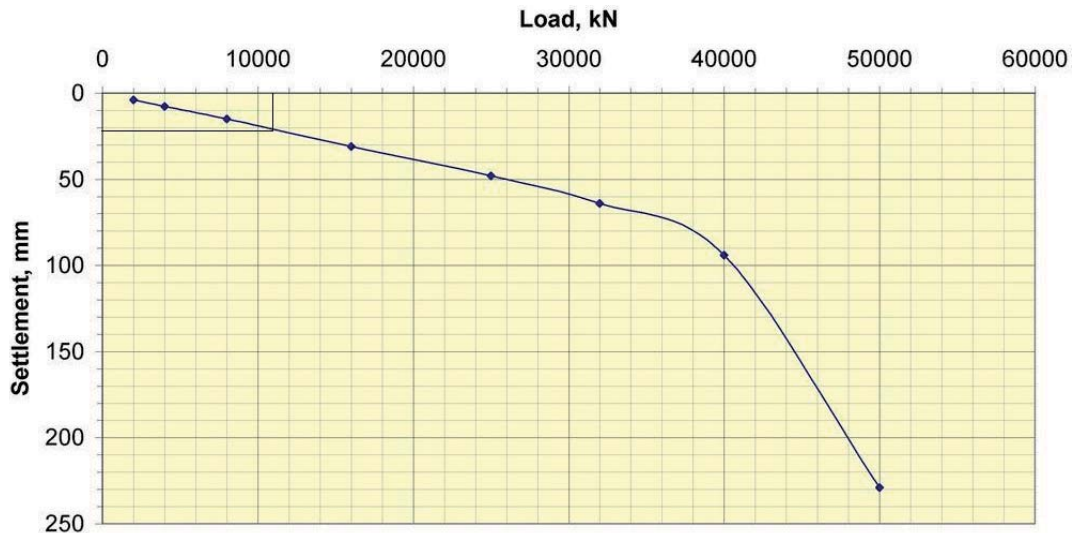
Fig. 3 Predicted vertical load-deformation performance of the tested pile obtained by the PLAXIS 3D software
