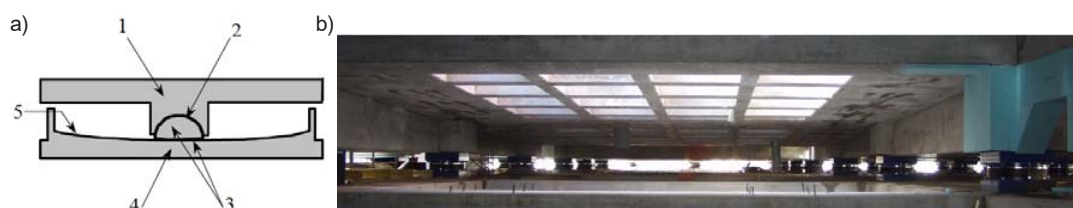
Fig. 2. PSB device (a): 1 — housing plate; 2 — articulated slider; 3 — sliding coating; 4 — concave plate; 5 — stainless steel concave surface; Installation of a PSB at a construction site (b)
