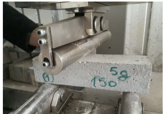
Fig. 7. Prismatic specimens of dimensions 7 × 7 × 28 cm for tensile strength testing
