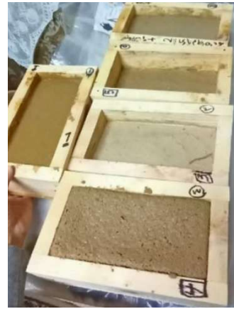
Fig 4. Five prepared brick samples (researchers' work)
