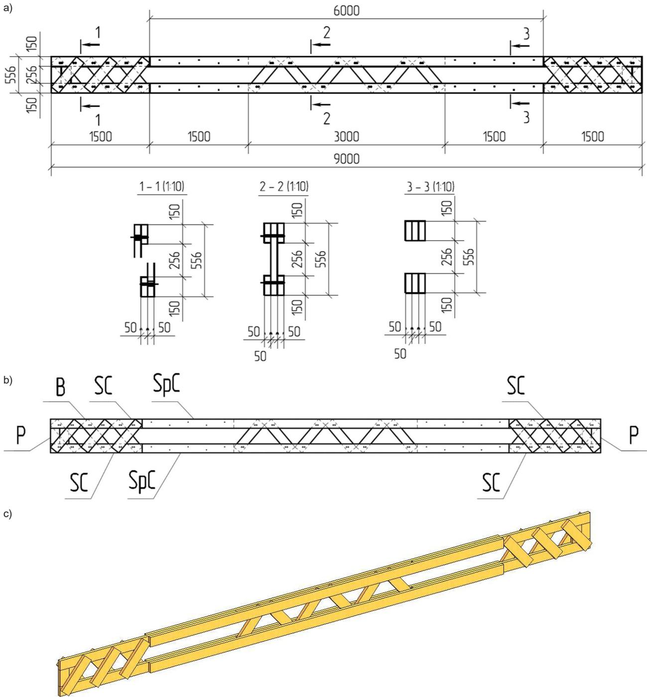
Fig. 1. Lattice girder truss: (a) geometric dimensions; (b) description of the beam elements; (c) 3D view.
