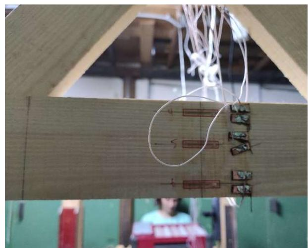
Fig. 3. Arrangement of strain gauges:
