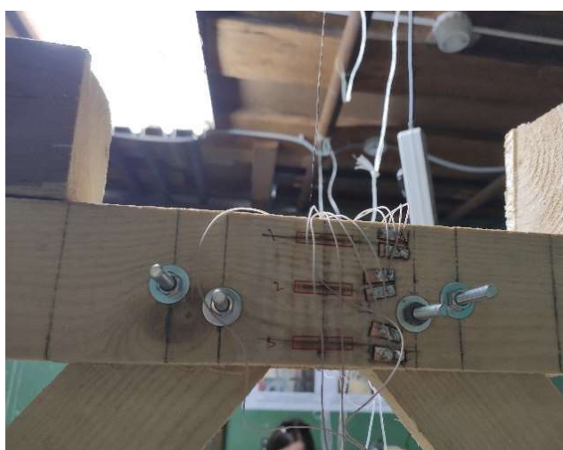
Fig. 3. Arrangement of strain gauges: a) in the middle of the structure span; b) on the upper and lower span chords, respectively
