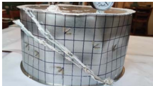
c) experimental model 2: buckling in the entire shell
