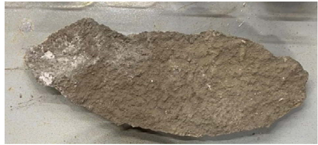
Fig. 6. Sample No. 1 of the plaster of the facade of the Yaroslavl Central Bank building
