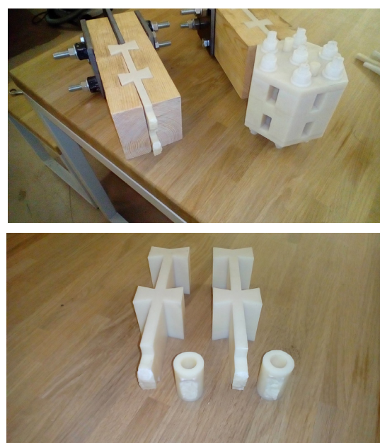
Fig. 10: a — the destroyed node, b — the destroyed elements of the node. Photo by D. Zhivotov
