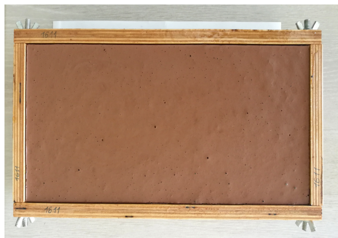
Figure 3. Appearance of the aerated clay mass made of Mix 1 during drying
