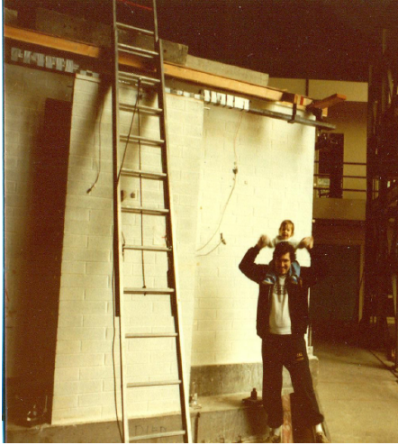
A Single-Story Masonry House on the EERC earthquake simulator facility
