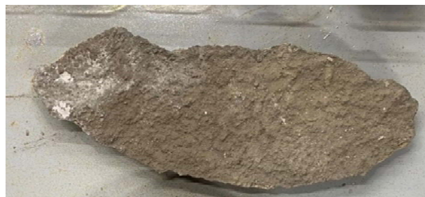
Fig. 6. Sample No. 1 of the plaster of the facade of the Yaroslavl Central Bank building
