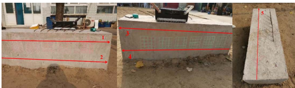
Fig. 3. Survey line arrangement of defects location on concrete specimen
