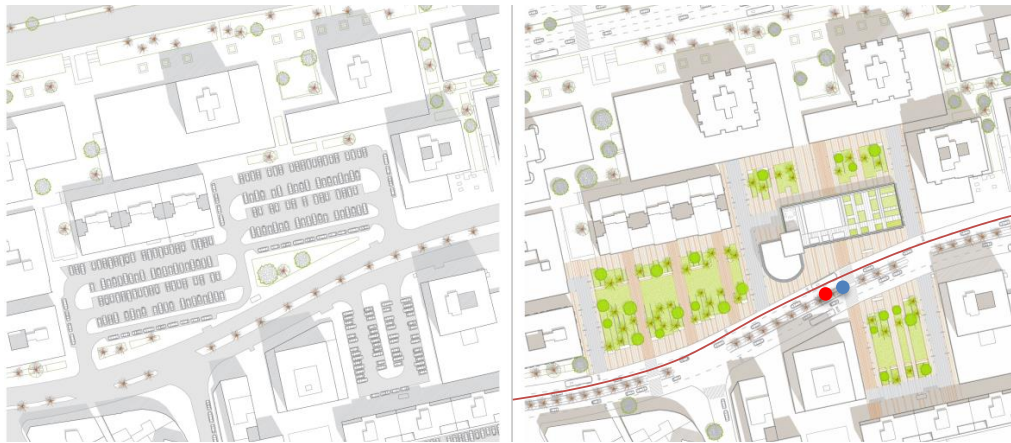
Fig. 6. Environmental recovery of 3660 m 2 as a result of eliminating the outdoor parking lots (left) after setting up the SMMN (right). Cycle lane (red line) and concentration of public transport: buses (red dot) and taxis (blue dot). Source: authors
