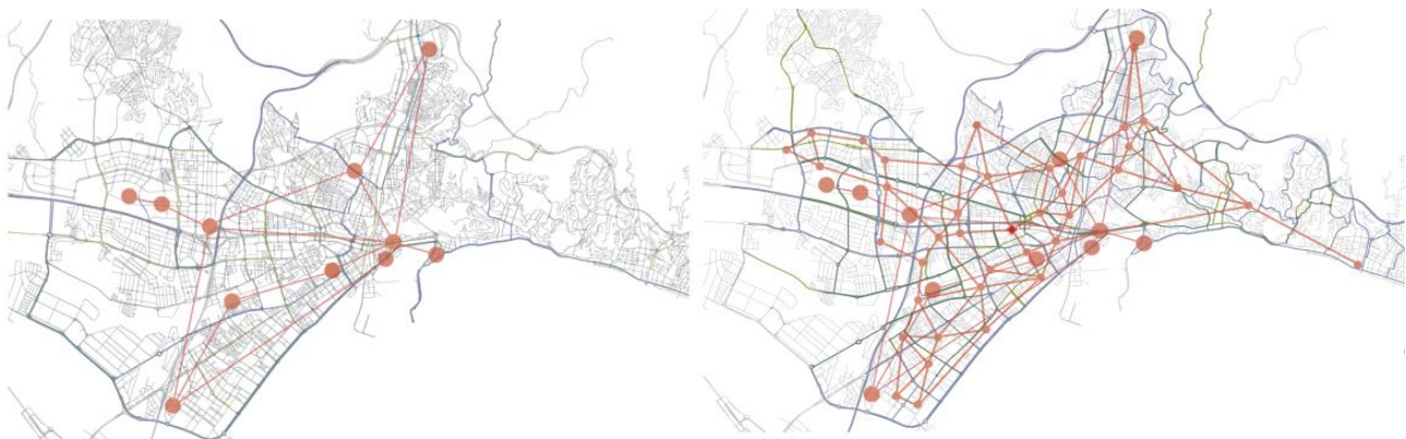
Fig. 11. On the left: primary system of large transport interchanges in Malaga; on the right: overlapping of the secondary system consisting of the SMMN network in different superblocks. Source: authors
