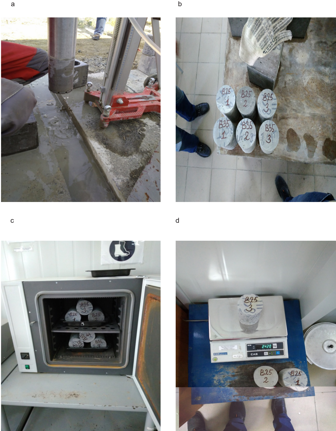
Fig. 2. Testing of the core samples to determine water absorption in B25 and B35 concretes: a — a portable SOLGA SDR 450 diamond drill rig; b — marking of the core samples; c — drying of the samples to determine the moisture-free mass (in a SNOL 58/350 laboratory low-temperature electric drying oven); g — weighing of the core samples after drying to determine the moisture-free mass (MWP-3000H laboratory balance, verification certificate No. VG-000000401 dated May 02, 2019)
