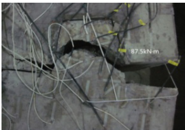
Fig. 15. Failure mode in the full-scale test
