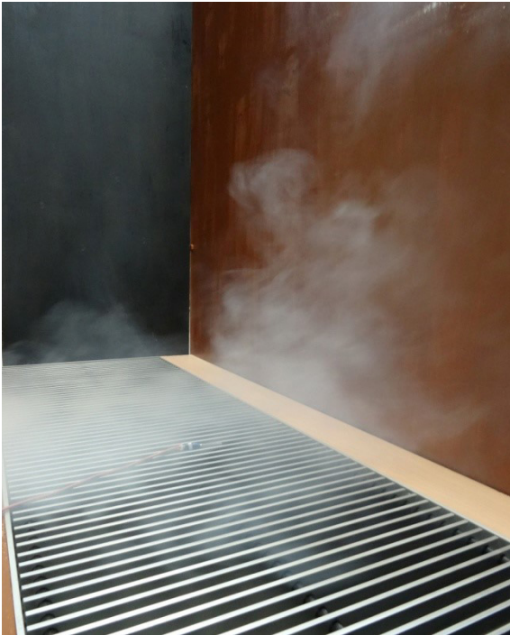
Fig. 3. Visualization of air flows (by smoke screening) at location of the heating element at a box wall from the room side (option 1); convector at a distance of 100 mm from the wall (glazing)
