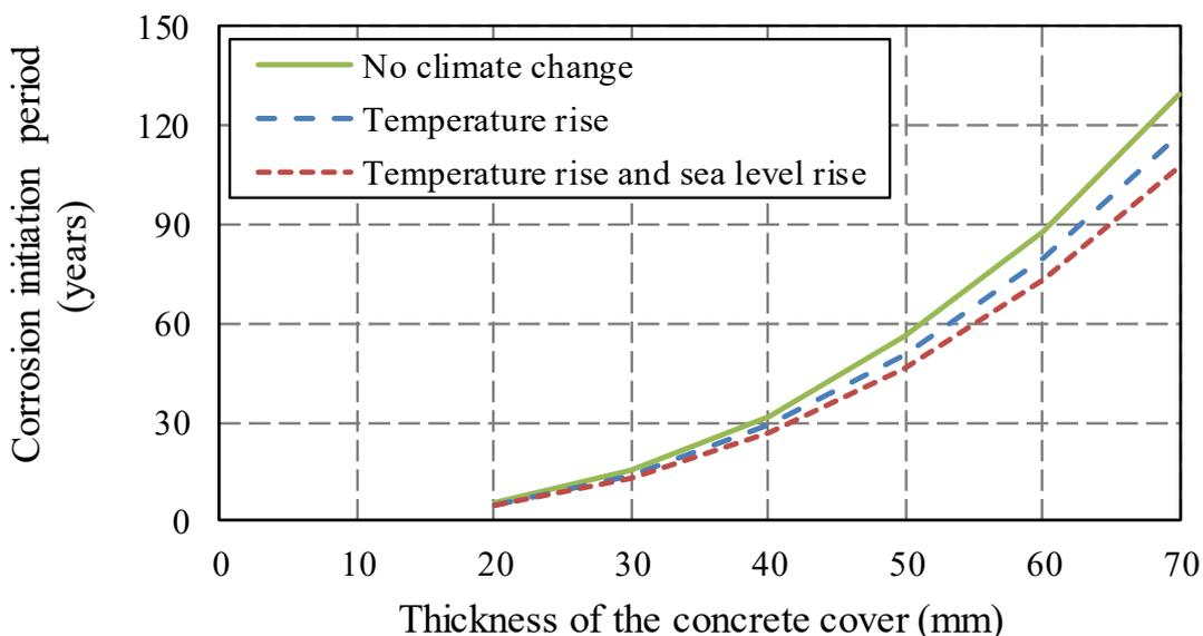
Figure 4. Corrosion initiation time for a structure with concrete C2
