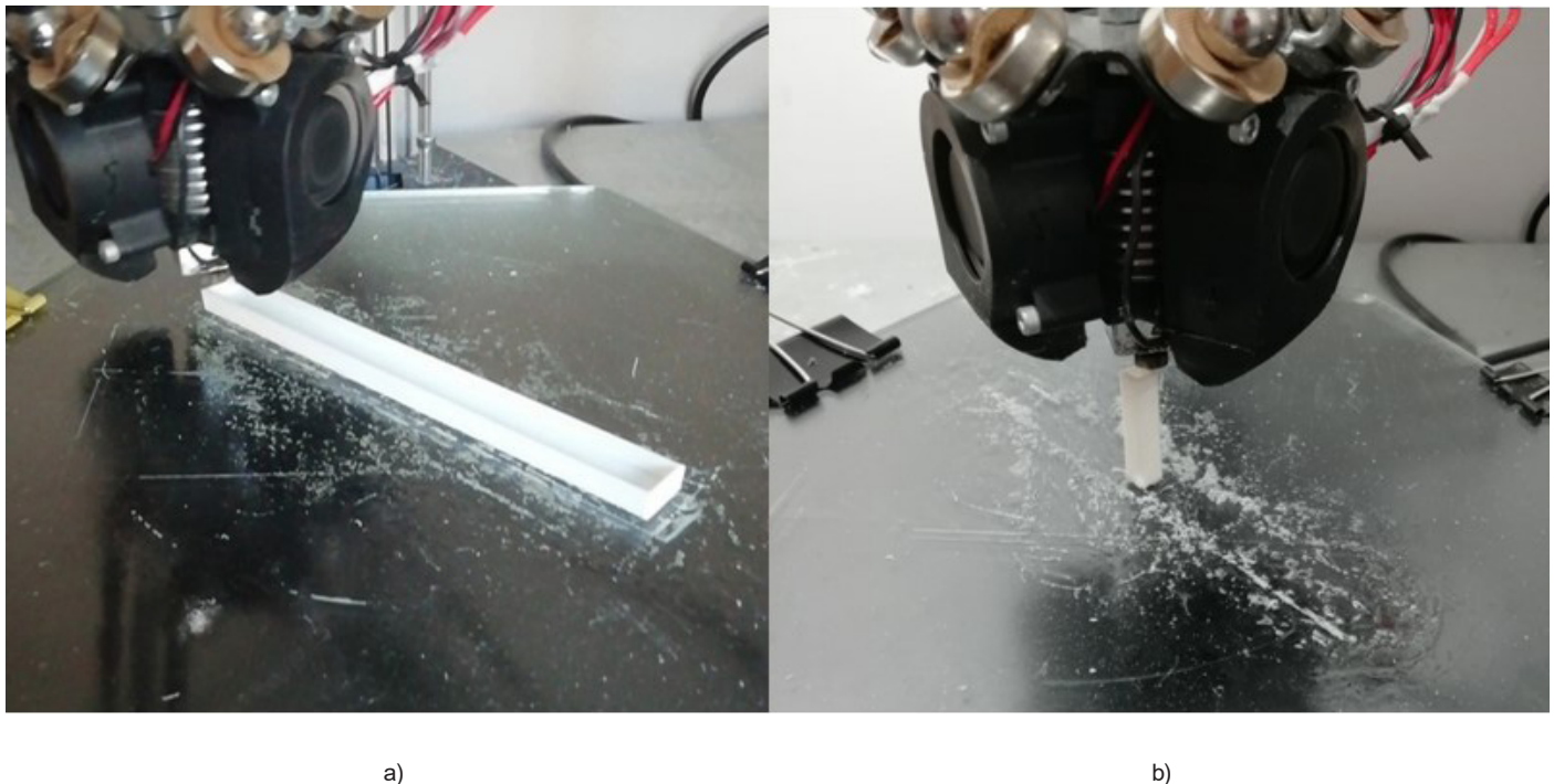
Figure 1. Arrangement of samples on the table of a 3D printer: horizontal (on the left), vertical (on the right)
