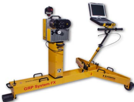
Fig. 4. GRP5000 tunnel scanning system
