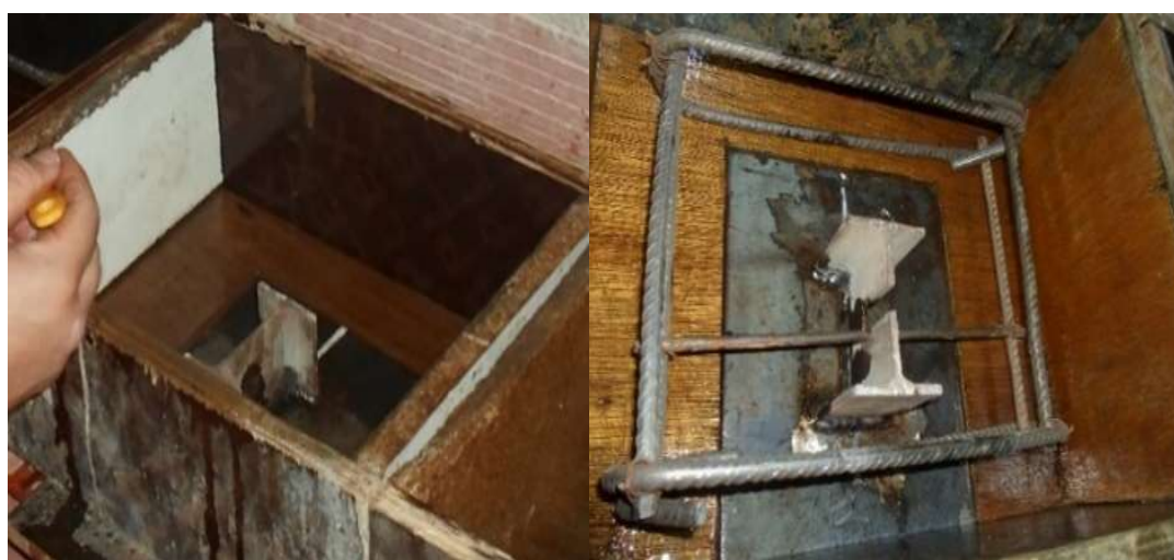
Fig. 3. Push-out specimen preparation
