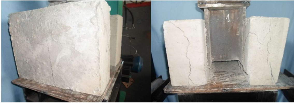
Fig. 8. Failure of IPE6C, IPE8C, IPN6C and IPN8C specimens
