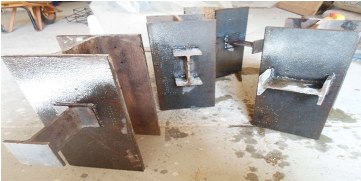
Fig. 1. IPE shear connectors studied in different orientations (Farid and Boutagouga, 2021)
