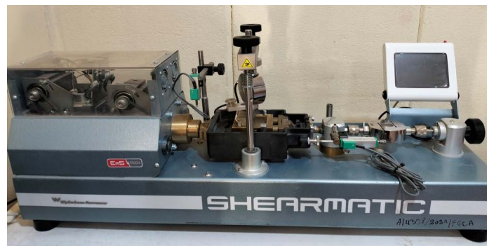
Fig. 5. View of the direct shear apparatus
