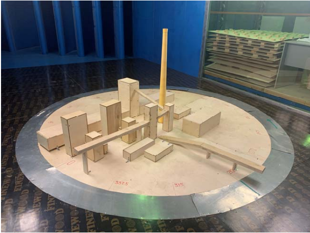
Fig. 6. Model of the chimney as part of the coke oven complex, scale 1:125
