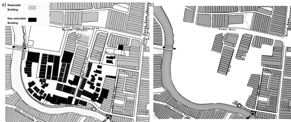
Fig. 9: a) status of structures after analysis, b) KJ after removal of dilapidated structures
